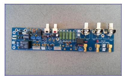
The built in control unit is a new development, comprising all the necessary circuits to control the transverter, regulate the cooling fan's speed, a 20dB/5Watt RF attenuator, as well as the jumper tabs to configure the transverters to the different HF radio types. The unit contains also the RF VOX unit (don't use it to replace of PTT input!) to save the RX IF amplifier if you forget to connect the PTT cable.
