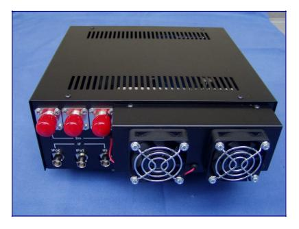
The transverters rear plate is accomodates the heat sink (for 50W version furnished with cooling fans, as standard) and the connectors as follows:
