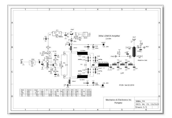
The input stage has a 6dB attenuator, followed by a 4:1 broadband transformer. The idle current of the LDMOS is set by potmeter P1.
