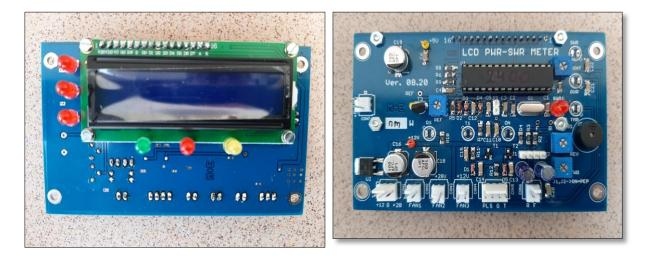
The display PCB contains a 2-line LCD display with associated circuitry, and the FWD and REV potentiometers for PWR scale calibration.
