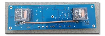
The RF relays are high-performance Finder PCB signal relays mounted on the back of the panel. The input and output cables to the power amplifier module are each connected to an SMA socket. The protection circuit is solved with a fast operational amplifier and thyristors. The protection circuit performs 4 functions.
