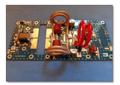
The 6dB/50W attenuator we placed at the input of the amplifier. This attenuator provides a constant load to the driver unit.
