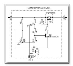
When the amplifier is on and the STBY/OPR switch is on OPR, the FET switches the DC voltage to the pallet.
