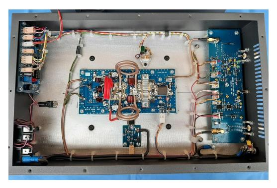
The complete pallet is located in the middle of the heat sink. The pallet is directly cooled by 2pcs 60x60mm fans attached to the bottom cover.
