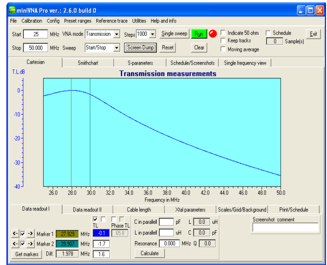
Characteristics of 28MHz IF amp. & LPF filter
