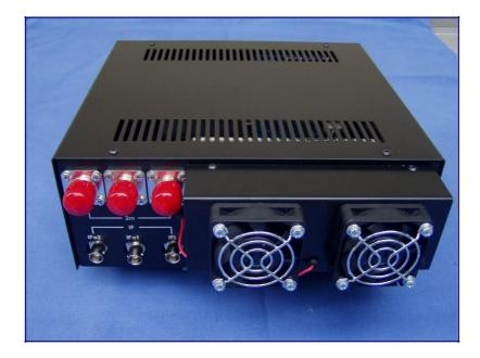
The transverters rear plate accommodates the heat sink and the connectors as follows:
