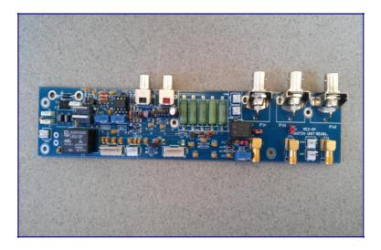
The built in control unit is a new development, comprising all the necessary circuits to control the transverter, regulate the cooling fan's speed, a 20dB/5Watt RF attenuator, as well as the jumper tabs to configure the transverters to different HF radio types. The unit contains also the RF VOX unit (don't use it to replace of PTT input!) to save the RX IF amplifier if you forget to connect the PTT cable.
