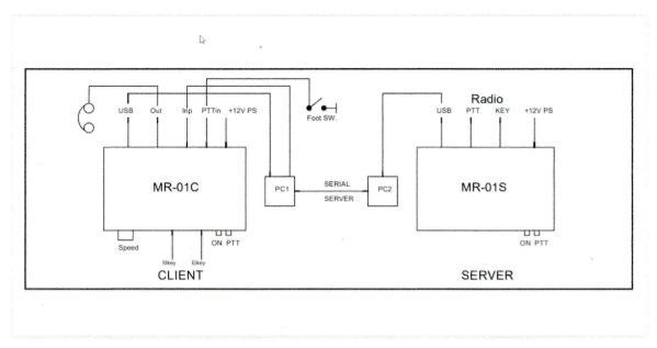
**Usage of SM7LCB serial server to the keyer:** (other similar serial server program is usable) The SSB mode works seamlessly with a laptop or PC for example, and the Remote station can be remote controlled as described above.
